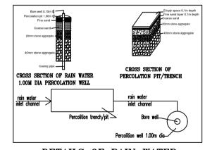
DETAILS OF RAIN WATER **HARVESTING STRUCTURES**
